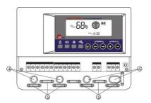
Cable come from the below®: cut the left and right plastic flaps using an appropriate tool (e.g. knife) and break them out of the case.
