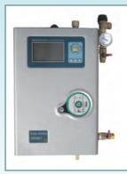
Circulation Pump: (WILO) 220V50HZ,RS15/6 Max flow:2.5(t/h) Max lift: 5.5m Suitable power of electrical heater:1pc,<1500W INPUT: One Sensor for collector(pt1000,probe≤ 500°C,Silicon cable≤280°C) Two Sensors for tank (pt1000,probe≤135° C,pvc cable≤105°C) Ambient temperature: -10~50°C
